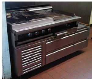
Commercial gas oven w/griddle
