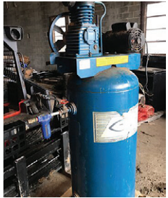
Vertical Air Compressor
