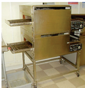
Impinger 18" stacked elec. conveyor ovens
