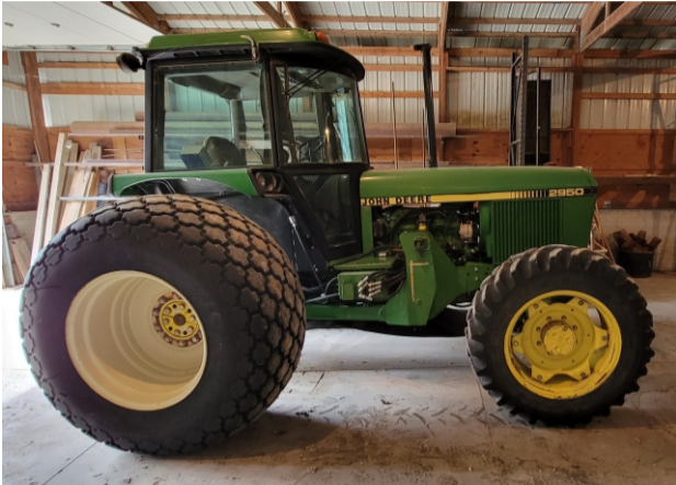
1983 John Deere 2950 Tractor FWA 4WD 5281 hours, #495876L, custom windrow panel, With 260 Loader, Firestone 30.5.5L-32 turf tires
