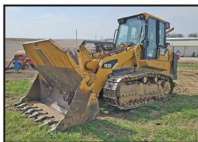
D04311 '09 CAT 963D track loader
