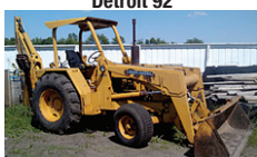
1974 JD backhoe, 18"x24" buckets w/JD 510 loader bucket (will dig a 19' hole)
