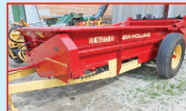
NH 520 SPREADER W/GATE, TOP BEATER, HYD VARIABLE DRIVE
