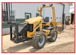
**2011 Vermeer RTX750**, 4WD, 4-wheel steer, 10" wide cut, full cup cutters, lays up to 6" foam tile, detachable tile spool, detachable boot, winch, light package, foam filled tires, can be used as trencher only, 211 hrs., Location: Odebolt, IA 51458, Representative DeWayne Ricklefs (712) 830-9105
