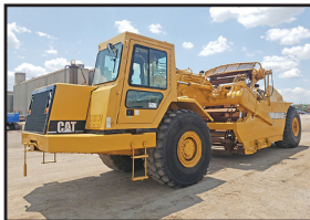
DP8075 '06 CAT 615C elevating scraper
