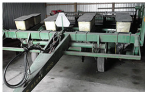
JD 7000 8 row 38's Planter! No-till ~ Heavy Down Pressure Springs, No-till Openers, Kinze Bean/Corn Meters
