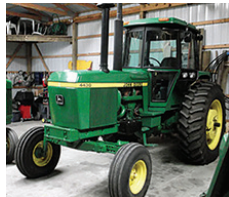
1977 JD 4430 Dsl Tractor! Quad Range, New 18.4x38's! New Cab Int. ~ Radio ~ Heat & Air S#0352898
