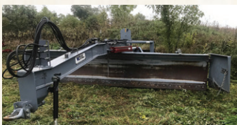
2012 B.I.L. HEAVY-DUTY PULL TYPE 14' BLADE BOX SCRAPER
