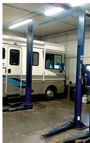
9,000 lb hoist (car lift)
