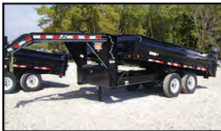
PJ D7 14' DUMP, GOOSENECK, 2-7K AXLES, 2 WAY GATE
