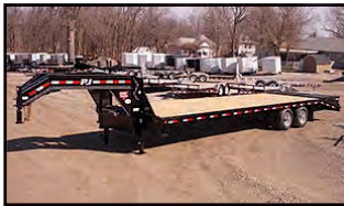
PJ FD 32' CLASSIC FLAT DECK W/DUALS, 2-10K AXLES, 5' DOVETAIL, 3 FLIP OVER RAMP
