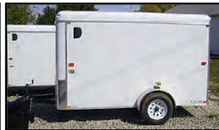
H&H CA 6x12, SINGLE AXLE, 72" WALL, ROCK GUARD, RAMP DOOR
