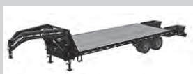
PJ FD Classic Flat Deck w/Duals 25'-36' w/2-10K Axles 5' Dovetail 3 Flip over Ramps
