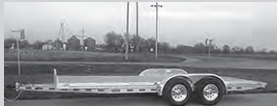
ZIMMERMAN ALUM COMBO CARHAULER 16', 18' & 20', Steel Frame w/2-5,200# Axles or w/2-3,500# Axles, Dovetail Rear Pull Out Ramps
