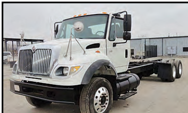
2005 IH 7600 Cat C-11, 305HP, 10 Spd., Air Ride, 12K Frt, 40K Rears, 270" WB, 195" C/A, Alum Wheels, Tire 22.5 85%, 522K Miles $29,500
