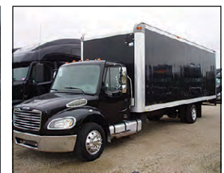
2005 Freightliner M2106 Medium Duty, M Benz 906, 190HP, Auto-Allison Trans, 4.63 Ratio, 254" WB, 19.5 Tires, Alum Wheels, 26' Van Box w/Pull Out Wall Up Ramp, Air Ride Suspension, Air Brakes, GVWR 26,000
