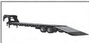
2015 PJ 32' Low Profile Deckover Flatbed w/Hyd Dovetail, Winch Plate, 2-10K Dexter Brake Axles, 20K GVWR, $12,750
