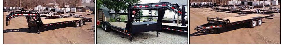
PJ FD 25' CLASSIC FLATDECK W/DUALS, TOOLBOX, 2-10K AXLES, 5' DOVE W/3 FLIPOVER RAMPS, RAMP SUPPORT ARMS PJ B6 22'x6" CHANNEL SUPER WIDE, GN, TOOLBOX, 2-7K AXLES, 2' DOVE, 5' FOLD UP RAMPS PJ F8 8' I-BEAM DECKOVER, 22', 2-7K AXLES
