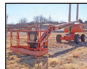
IS9447 '07 JLG 460SJ boom lift
