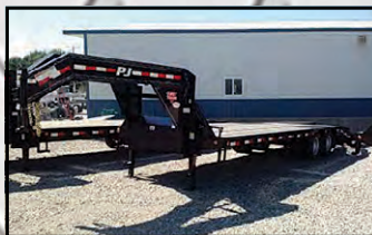
PJ LD 32' LOW PRO FLAT DECK W/DUALS, 2-10K OIL BATH AXLES, 2-DROP LEG JACKS
