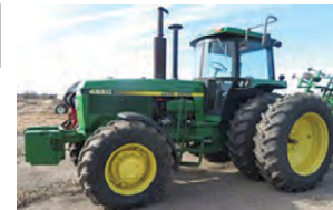
1983 JD 4650 FWA (mechanical FWD, 16x9xR28, 18x4x42, Trimble easy guide system, 7917 hrs)
