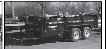
PJ D7 14' TANDEM AXLE DUMP, 2-7K AXLES, SPLIT SPREADER GATE, TARP KIT, SCISSOR LIFT
