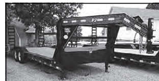
PJ B6 22' CHANNEL SUPER WIDE, GOOSENECK, TOOLBOX, 2-7K AXLES, 2' DOVETAIL, 5' FOLD UP RAMPS
