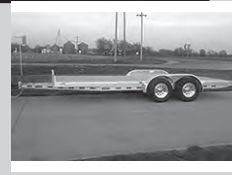
ZIMMERMAN ALUM COMBO CARHAULER , 16', 18' & 20' Steel Frame w/2-5,200# Axles or 2-3,500# Axles, Rear Pull Out Ramps
