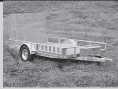
ZIMMERMAN ALUM COMBO UTILITY 12x77, Steel Frame w/1-3,500# Axle, Rear Gate, Side ATV Ramps
