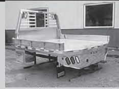
ZT FLATBEDS Steel Frame Alum Body w/B&W GN Rear Receiver Hitch All LED Lights
