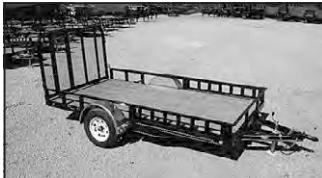
PJ U7 12'x77" CHANNEL UTILITY, 1-3,500# AXLE, STRAIGHT DECK W/4' FOLD UP GATE, SIDE ATV RAMP
