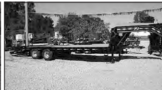
PJ FD 25' CLASSIC FLATDECK W/DUALS, TOOLBOX, 2-10K AXLES, 5' DOVETAIL, W/3 FLIPOVER RAMPS
