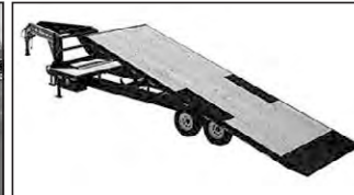
PJ T9 29' HD DECK OVER TILT, 2-7K AXLES, 2-DROP LEG JACKS, ELECTRIC BREAK AWAY KIT
