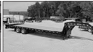
PJ FD 28' CLASSIC FLATDECK W/DUALS, 2-10K AXLES, 5' DOVE, 3 FLIP OVER RAMPS, COLD WEATHER HARNESS
