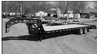
PJ FD 30' CLASSIC FLATDECK W/DUALS, 2-10K AXLES, SUPER SINGLE, 5' DOVE, 3 RAMPS, 72" AXLE SPREAD
