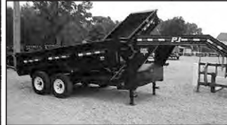
PJ D7 14' TANDEM AXLE DUMP, GOOSENECK, 2-7K AXLES, SPLIT/SPREADER GATE, TARP KIT
