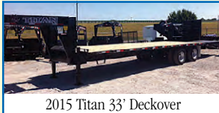
2015 Titan 33' Deckover Flatbed, 20K GVWR, 28' Deck w/5' Dovetail, Center Pop Up, Dual Jacks, Spare Tire & Wheel, Gray/White, $9,800
