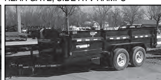
PJ D7 14' TANDEM AXLE DUMP, 2-7K AXLES, SPLIT SPREADER GATE, TARP KIT, SCISSOR LIFT
