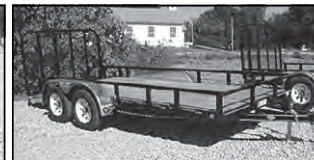
PJ U8 83" CHANNEL UTILITY, 16', 7,000# GVWR, 83" WIDE DECK, REMOVABLE ALUM TREAD PLATE FENDERS, REMOVABLE SIDES
