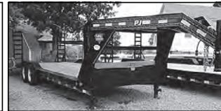
PJ B6 6" CHANNEL SUPER-WIDE, 22' GN, 14,000# GVWR, 102" WIDE DECK, DRIVE OVER FENDERS, 6" CHANNEL FRAME
