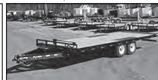
PJ T8, DECKOVER TILT, 22', 14,000# GVWR, 4' STATIONARY DECK ON 26', 8"x10" I-BEAM FRAME & TONGUE
