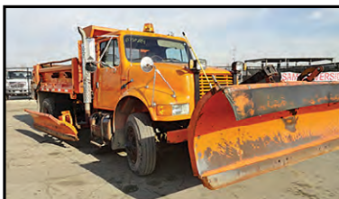
1994 IH 4900 10' Dump Box, Sander, DT-466 230HP, Auto, 11 Ft Frt Snowblade, 8 Ft Wing Blade, 170" WB, 11R22.5 Tires, 160,785 Miles, $10,900
