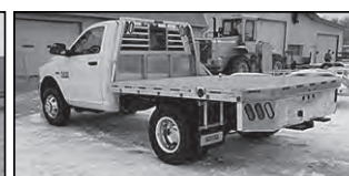
ZIMMERMAN ALUM COMBO ALUM FLATBED, STEEL FRAME ALUM BODY W/B&W GN HITCH, REAR RECEIVER HITCH, ALL LED LIGHTS, BUILT TO SUIT
