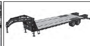
PJ LD LOW PRO FLAT DECK W/DUALS, 32', 22,400 GVWR, 10K-16K AXLES AVAILABLE, ULTRA LOW 33" DECK HEIGHT, 12"x19" I-BEAM MAIN BEAM
