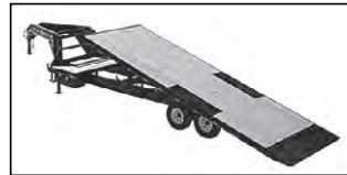
PJ T9 HD DECKOVER TILT, 29', 15,680# GVWR, 24" DECK, 12"x14" I-BEAM FRAME, 102" WIDE DECK, SCISSOR HOIST STANDARD, GN COUPLER STANDARD
