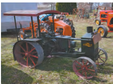
Rumley Oil Pull Tractor Homemade, 3.5 hp International Engine/Transmission
