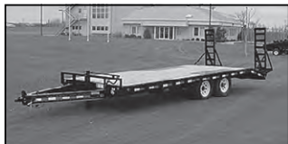
PJ F8 8" I-BEAM DECK OVER, 22', 2-7K AXLES
