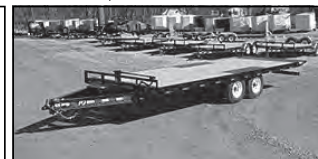
PJ T8 DECK OVER TILT, 22', 2-7K AXLES, 4' STATIONARY DECK 8x10 I-BEAM FRAME & TONGUE
