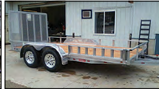
Zimmerman Utility 77x14, LED Lights, ATV Ramps, 4' Spring Assist Gate, 2-3,500# Axles w/Brakes
