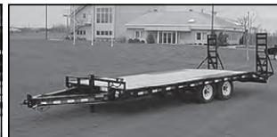
PJ F8 8" I-BEAM DECKOVER, 22' 2-7K AXLES
