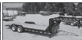
PJ CC 22'x24' 6" CHANNEL EQUIPMENT, GN, 2-7K AXLES, REMOVABLE FENDERS
