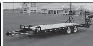
PJ F8 22'x24' 8" I-BEAM DECKOVER, 2-7K AXLES
