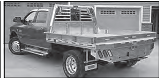
ZIMMERMAN ALUM COMBO FLATBED, STEEL FRAME ALUM BODY W/B&W GN, REAR RECEIVER HITCH, ALL LED LIGHTS
