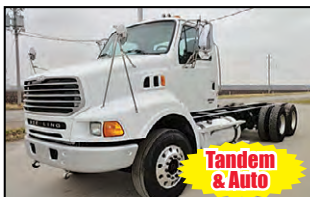
2006 Sterling 9500, Tandem Cab & Chassis, Mercedes 460HP, Allison 4560 6 Spd, 14,600 Lbs Frt, 40,000 Lbs Rear, 54,600 GVW, Long WB, PTO, Nice Clean Truck, Ready to Go
