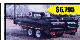
PJ D8 14' DECK OVER DUMP, 2-7K Axles, Side Dump, Scissor Hoist
