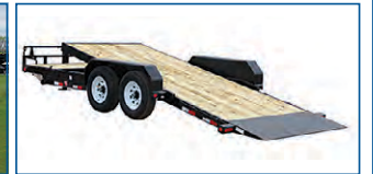
PJ T6 20' & 22' 6" CHANNEL EQUIPMENT TILT, 2-7K AXLES, STAKE POCKETS & RUB RAIL
