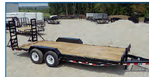
PJ CC 20' & 18' 6" CHANNEL EQUIPMENT, 2-7K AXLES, REMOVABLE FENDERS
