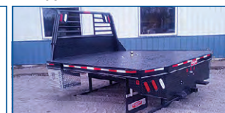
ZIMMERMAN STEEL FLATBED, W/B&W HITCH, REAR RECEIVER HITCH, ALL LED LIGHTS
