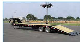
PJ FY 30' HYDRAULIC DOVETAIL, 2-10K AXLES
