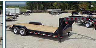
PJ CC 22' & 24' 6" CHANNEL EQUIPMENT, GOOSENECK, 2-7K AXLES, REMOVABLE FENDERS
