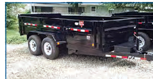
PJ D7 14' TANDEM AXLE DUMP, 2-7K AXLES, SPLIT/SPREADER GATE, TARP KIT, SCISSOR LIFT
