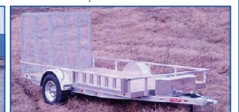
ZIMMERMAN ALUM UTILITY STEEL FRAME ALUM BODY, 1-3,500#AXLE, REAR GATE, SIDE ATV RAMPS
