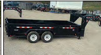
PJ DJ 16'x83" LOW PRO XL DUMP , 2-7K AXLES, GN, SPLIT/SPREADER GATE
