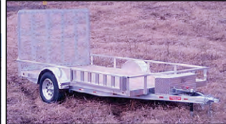
ZIMMERMAN ALUM COMBO UTILITY , 12'x77" STEEL FRAME ALUM BODY, 1-3,500# AXLE, REAR GATE, SIDE ATV RAMPS
