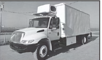
2006 International 4300, DT466 230HP, Auto, 12K Frt, 21K Rear, 33,000 GVW, Air Brakes, 20 Ft Reefer Body w/Side Door & Alum Lift Gate, 238" WB, 168" CA, 228" Cab to End of Frame, Tires 295/75R22.5 65%, 2-50 Gal Step Tanks, Just Off Lease, Clean Truck, Only 152,245 Miles, Will Sell w/Box for $21,900
