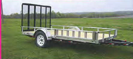
ZIMMERMAN 12'X77" Utility Alum Body, Steel Frame, 1-3,500# Axle, Fold up Gate ATV Ramps, LED Lights
