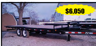
PJ T8 22' DECK OVER TILT, 2-7K AXLES, HYDRAULIC TILT
