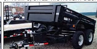
PJ D5 10'x60" UTILITY DUMP, 2-5K AXLES, SPLIT/SPREADER GATE, TARP KIT, SCISSOR LIFT
