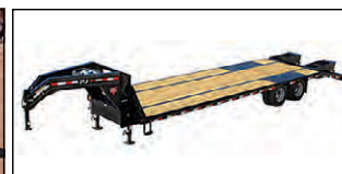
PJ LD 32' LOW PRO FLAT DECK W/DUALS 2-10K OIL BATH AXLES, 2-DROP LEG JACKS
