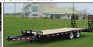
PJ F8 20' I-BEAM DECKOVER, 2-7K AXLES, 3' DOVETAIL, W/2 FOLD UP RAMPS, OR 22' W/STRAIGHT DECK
