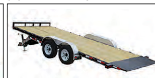
PJ TH 20' 83" HYDRAULIC QUICK TILT, 2-3,500# AXLES, DROP LEG JACK
