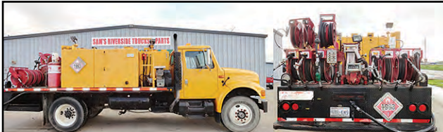
1992 International 4900 Lube Truck, DT-466 220HP, 7 Spd w/Overdrive Manual, 188" WB, 12K Fr, 23K Rear, Equipped w/Hyd Air Compressor, Hyd Generator, 800 Gallon Fuel Tank, Air Greaser, Five Storage Tanks For New Oil, One Storage Tank For Waste Oil, 1122.5 Tires 70%, 9,353 Miles, 8,516 Hrs., Nice Clean Truck, $29,900
