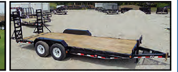
PJ 20' 6" CHANNEL EQUIPMENT CARHAULER 2-7K AXLES, DOVE-TAIL, STAND UP RAMPS
