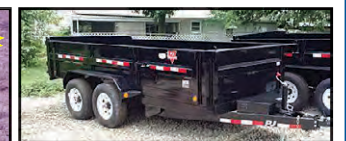
PJ D7 12'83" TANDEM AXLE DUMP, 2-7K AXLES
