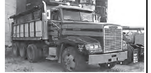
1990 Freightliner FLD120 855 Cummins, 9 Spd., 12K Front Axle, 40K Air Ride Rear w/3rd Axle, 15' Bed w/Roll Over Tarp $7,500
