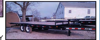
PJ T8 22' DECKOVER TILT, 2-7K AXLES, HYDRAULIC TILT
