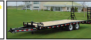
PF F8 22' 8" I-BEAM DECKOVER 2-7K AXLES, 2 STAND UP RAMPS
