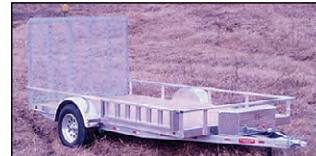
ZIMMERMAN ALUM COMBO UTILITY, 12'x77" STEEL FRAME ALUM BODY, 1-3,500# AXLE, REAR GATE, SIDE ATV RAMPS
