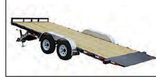
PJ TH 20' 83" HYDRAULIC QUICK TILT, 2-3,500# AXLES, DROP LEG JACK
