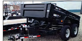
PJ D5 10'x60' UTILITY DUMP, 2-5K AXLES, SPLIT/SPREADER GATE, TARP KIT, SCISSOR LIFT
