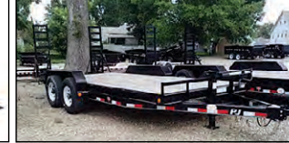
PJ CC 18' CHANNEL EQUIPMENT, 2-7K AXLES, 2' DOVE, 5' FOLD UP RAMPS, RUB RAIL
