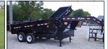
PJ D7 14'TANDEM AXLE DUMP, GOOSENECK, 2-7K AXLES, SPLIT/SPREADER GATE
