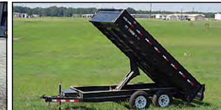
PJ D8 14' 96" DECKOVER DUMP, 2-7K AXLES, SPLIT/SPREADER GATE
