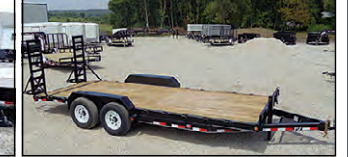
PJ CC 20' CHANNEL CUSTOM EQUIPMENT, 2-7K AXLES, 5' CHANNEL RAMPS
