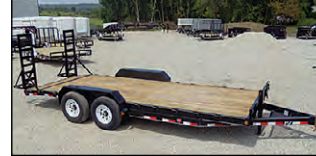
PJ CC 20' CHANNEL CUSTOM EQUIPMENT, 2-7K AXLES, 5' CHANNEL RAMPS
