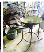
Lancaster #40 Blacksmith Forge
