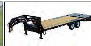
PJ LOW PRO FLAT DECK W/SINGLES (LS) 25', W/TOOLBOX, 2-7K AXLES, SLIDE IN RAMPS
