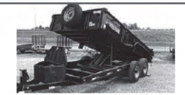
2013 Titan 82"x14" Bumper Pull Dump Trailer 14K GVWR, 2-7K Torque Flex Brake Axles, Dual Rear Gate, Goodyear 10 Ply Tires w/Spare, $7,550 $7,150
