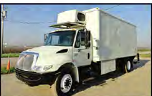
2006 International 4300, DT466 230HP, Auto, 12K Frt, 21K Rear, 33,000 GVW, Air Brakes, 20' Reefer Body w/Side Door & Alum Lift Gate, 238" WB, 168" C/A, 228" Cab to End of Frame, Tires 295/75R22.5 65%, 2-50 Gal Step Tanks, Just Off Lease, Clean Truck, Only 152,245 Miles, Will Sell w/Box for $21,900
