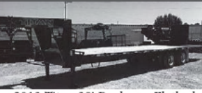
2013 Titan 30' Deckover Flatbed 24' Deck, 6' Wide Glide Dovetail 2-6'x48" wide Ramps, 2-10K Dexter Elec Brake Axles, Goodyear Tires w/ Spare, $9,200
