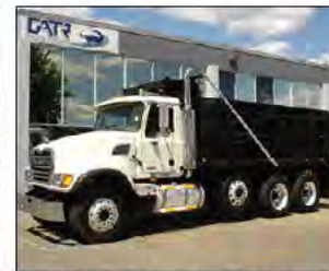
2006 Mack CV713 Mack Engine @ 427 HP, Allison Automatic 4500 RDS Series, Steel Dump Body, 370K Miles
