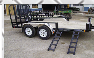
PJ UTILITY 83x14, Side Load Ramps, 4' Spring Assist Gate, 2-3,500# Axles
