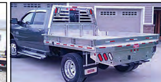
ZT ALUM FLATBED, STEEL FRAME, ALUM BODY, B&W GN & REAR RECEIVER HITCH, ALL LED LIGHTS
