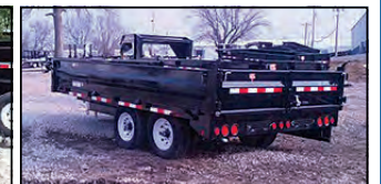
PJ 14' 96" DECKOVER DUMP (D8), 2-7K AXLES, 19" HIGH FOLD DOWN SIDES, 96" WIDE BED, SLIDE IN RAMPS
