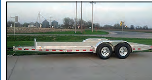
ZIMMERMAN ALUM COMBO CARHAULER, STEEL FRAME, ALUM BODY, 2-5,200# AXLES, PULL OUT RAMPS
