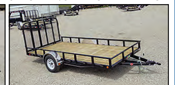
PJ 83" CHANNEL UTILITY (U8) 1-3,500# AXLE, REAR GATE SIDE ATV RAMP
