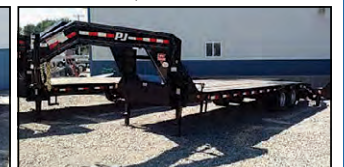
PJ 28' 30' 32' LOW-PRO FLATDECK W/ DUALS (LD) 2-10K AXLES, 5' DOVE W/3 FLIP OVER RAMPS
