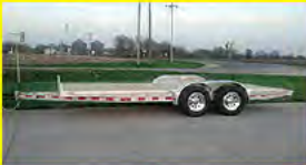
ZIMMERMAN ALUM COMBO CARHAULER, 16', 18' & 20' w/2-5,200# Axles or w/2-3,500# Axles, Dovetail Rear Pull Out Ramps
