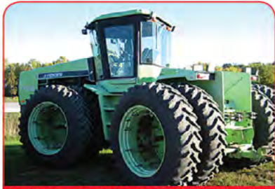
'86 Steiger CR 1225, 6400 Total Hrs., 18/42 Duals, 3306 CAT Set AT 280HP, 20 spd., PTO, Lots Of Work Done, $39,500
