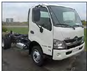
2013 Hino 195 19,500 GVWR, 210HP Hino Engine, Automatic Transmission, 138" WB, Will Hold A 16' Body
