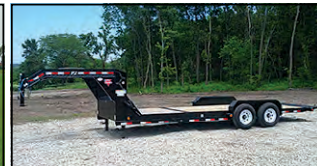
PJ 6" CHANNEL EQUIPMENT TILT (T6) 22' GN 2-7K AXLES
