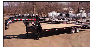
PJ CLASSIC FLATDECK W/SINGLES (FS) 33' & 28', 2-7K AXLES, 102" WIDE DECK, 2-DROP LEG JACKS, FRT TOOLBOX
