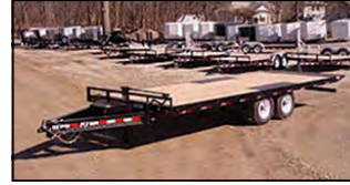
PJ 8' I-BEAM DECK OVER (F8) 20', 22', 24', 2-5,200# AXLES 96" WIDE DECK
