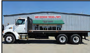
2004 Sterling L8500 CAT C-7, 210HP, 8LL Trans, Tandem Axle, Hendrickson Susp., 21" Steel Flatbed, 22.5 Tires 80%, 136,529 Miles, Nice Clean Truck, $16,900
