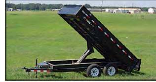
PJ 96" DECKOVER DUMP (D8), 14' 2-7K AXLES, 2-WAY GATE (BARN DOORS & SPREAD GATE), TOOLBOX, SCISSOR LIFT
