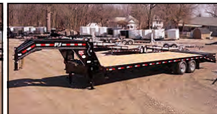
PJ CLASSIC FLATDECK W/DUALS (FD) 25', 28', 30', 40', 2-10K AXLES, 2-DROP LEG JACKS, FRT TOOLBOX
